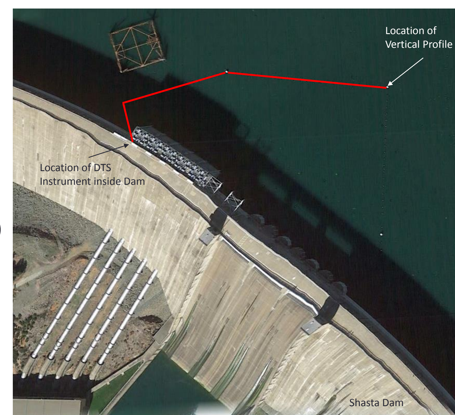
Figure 3: Plan view of cable deployment at Shasta Lake. Red line indicates path of cable.
