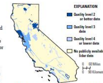
Figure 1. Map of California showing the areal extent and quality levels of planned and existing publicly available light detection and ranging (lidar) data in August 2013. Quality level 2 or better lidar data meet 3DEP requirements. See table 2 for quality level information.
