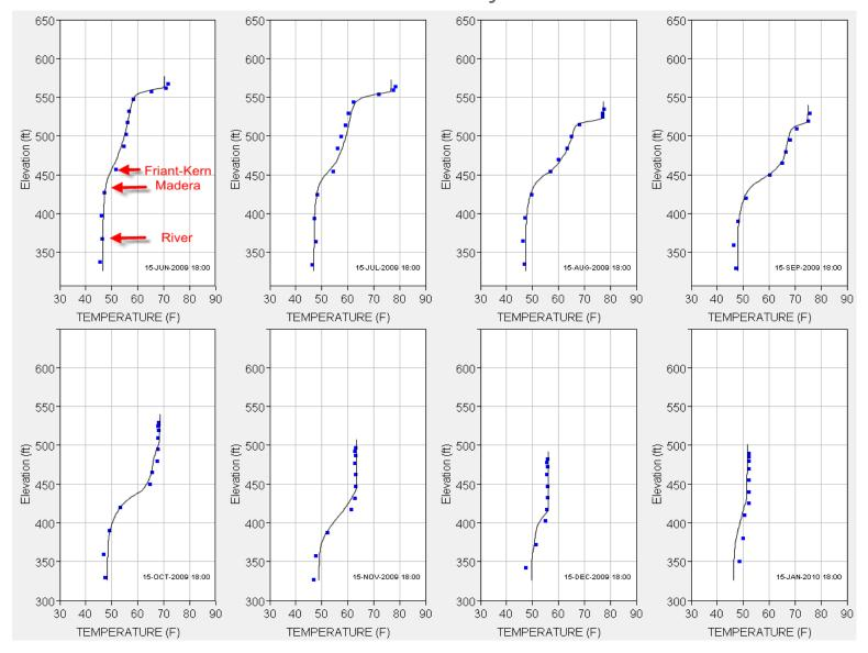
Impact of Hydrology on Cold Water Resource - Lower Runoff Volume
